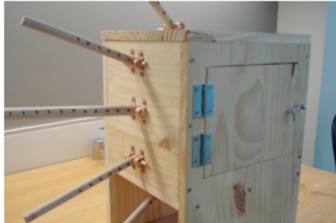
Figure 5. Raised wooden box structure showing the 5 wooden dowels and the hinged-door system.
