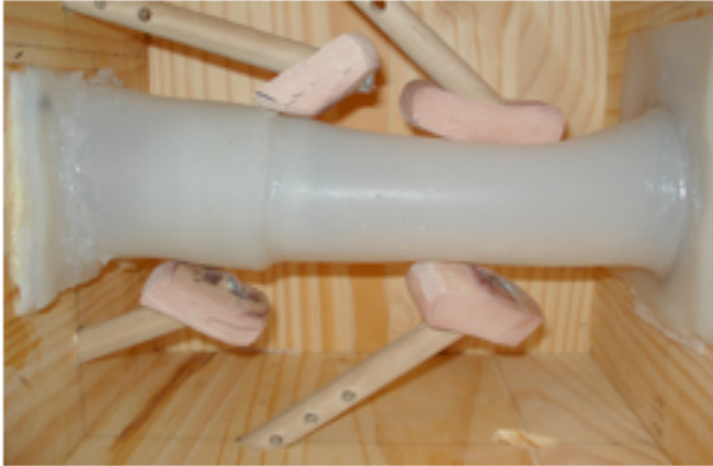
Figure 6. Silicone tube attached with Velcro™ to the front and back of the model. Wooden dowels with Sculpey™ clay attached to them move through the 5 holes positioned at the top, bottom, and back of the model.
