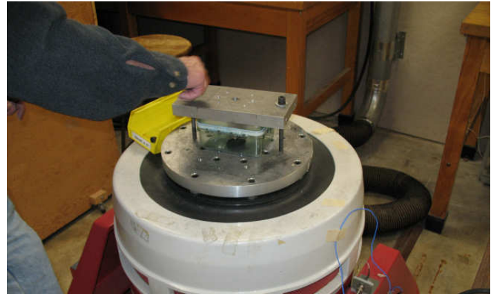
Figure 17- Shock table used to execute mock transportation vibration testing. Shown is our chamber on top
