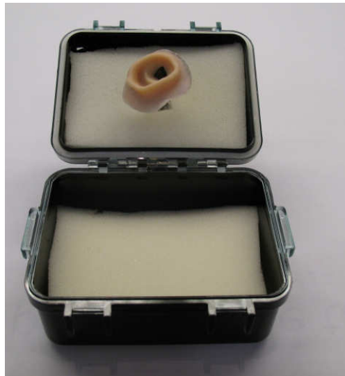
Figure 14: Picture of eye design with extra layer of foam in bottom of chamber with eye attached to suction cup stabilization stem on top of chamber.
