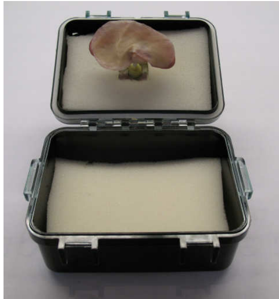
Figure 16: Picture of eye design with extra layer of foam on bottom of chamber with ear attached to putty mold stabilization stem on top of chamber.
