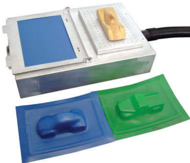
Figure 4. Vacuum molding machine which heats the plastic and vacuum forms it
