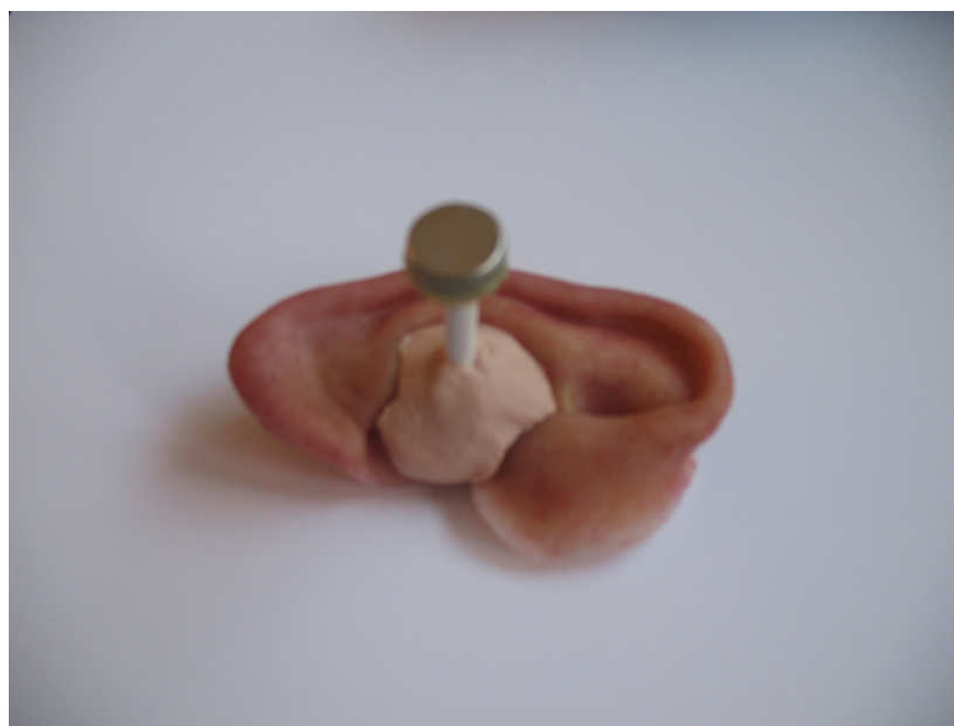
Figure 15: Picture of eye design with extra layer of foam on bottom of chamber with ear attached to putty mold stabilization stem on top of chamber.
