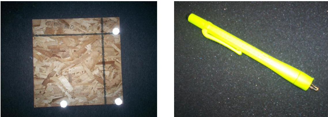
Figure 7: The ground square we constructed with homemade reflective markers (left), and the converted LED pen (right).
