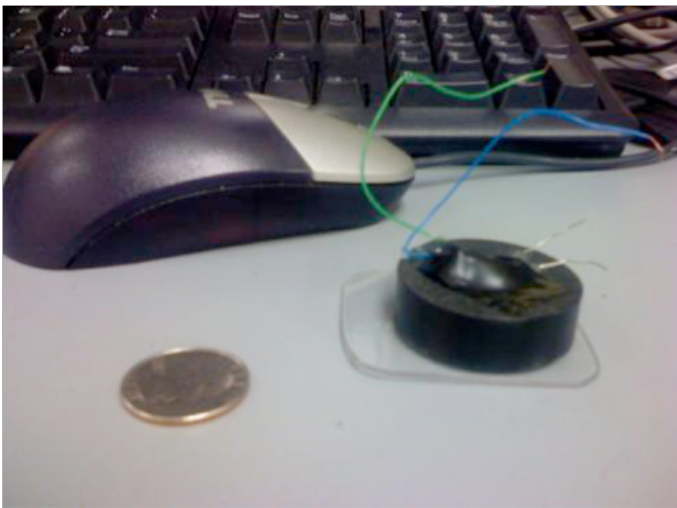
Figure 3. Image of the sensor and housing design developed by the fall 2007 design team. (Ginter, Ho, Kurkiewicz, & Yuen, 2007).
