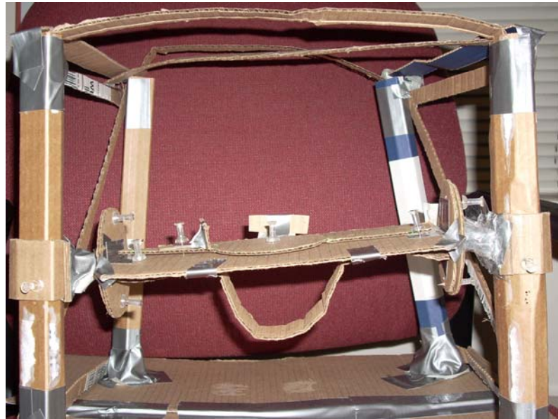
Figure 4: Front view of the model with bite block and adjustable system in the foreground. It includes vertically moving collars, rotating plate for pitch, and rotating disk for yaw adjustments.
