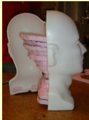
Fig. 4 Model cutaway showing foam cross-section assembly
