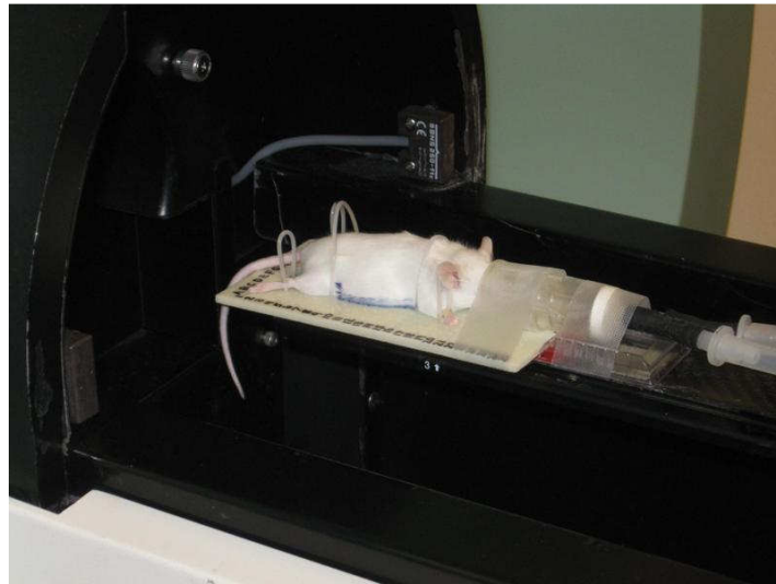
Figure 30: In order to test our device, a mouse was positioned on our board and a CT scan was performed. This process was repeated with the same mouse eight times.
