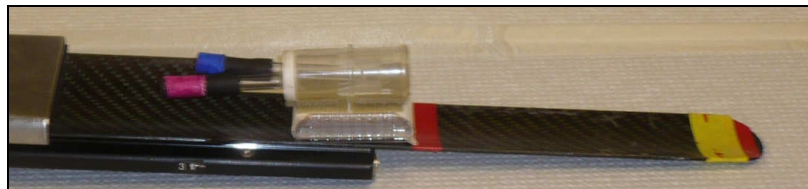
Figure 1: The animal's limbs are secured with tape during a scan. This method makes it difficult to reposition the mouse for consecutive scans.
