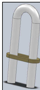
Figure 23: An orthodontic rubber band is glued 3/16" above the bottom of each peg.
