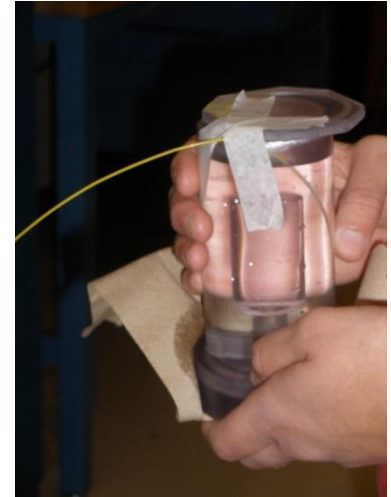
Figure 7 - Temperature testing with fiber optic probe.
