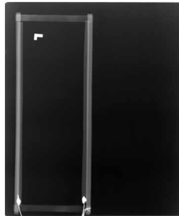
Figure 16: X-ray image used to quantify radiolucency. Notice how little the device (enclosed by busbars) attenuates the X-ray beam.
