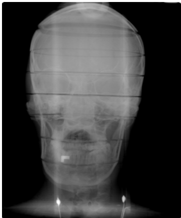
Figure 15: X-ray image of device and phantom. Although the busbars are visible, that was to be expected and will be accounted for by designing the device such that the busbars are outside the exposure field.
