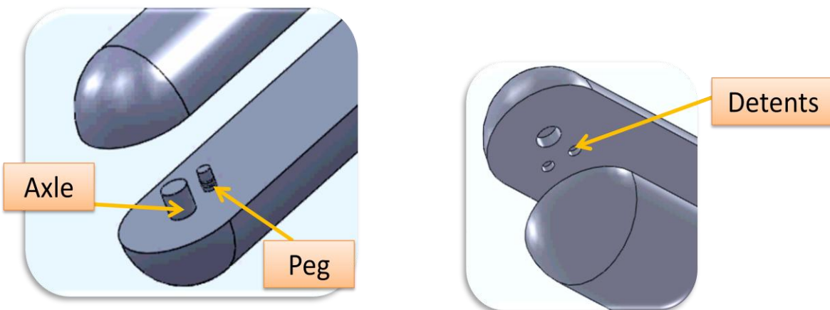
Figure 11 – SolidWorks image of the detent hinge liver retractor. A retractor arm is pictured left with a spring-coupled peg that fits into one of two detents in the base rod pictured right.
