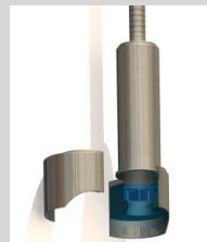
Figure 3: Metal Design. Failed because it was Heavy.
