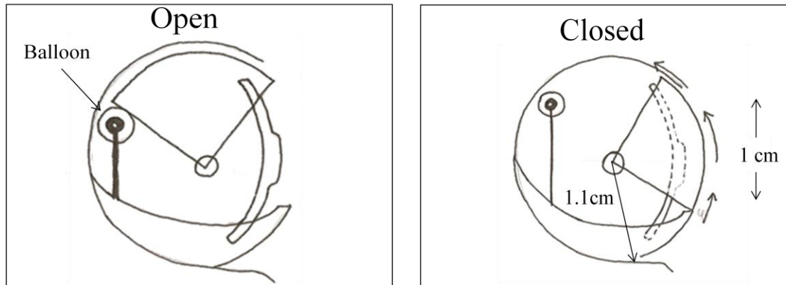
Figure 6. Diagram of the pneumatic design alternative, which utilizes air pressure stored in a closed system to inflate a catheter, and trigger a blink. External controlling device not shown.
