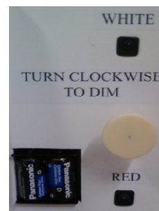
Figure 9: View from behind board (switches, potentiometer knob, and batteries)
