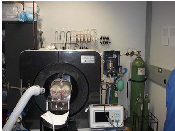
Figure 1: This picture shows four rats in the PET scanner at the client's laboratory. The rats are orientated in a two by two square. Picture taken from last semester's design team's final paper.
