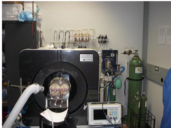
Figure 1: This picture shows four rats in the PET scanner at the client's laboratory. The rats are orientated in a two by two square [1].
