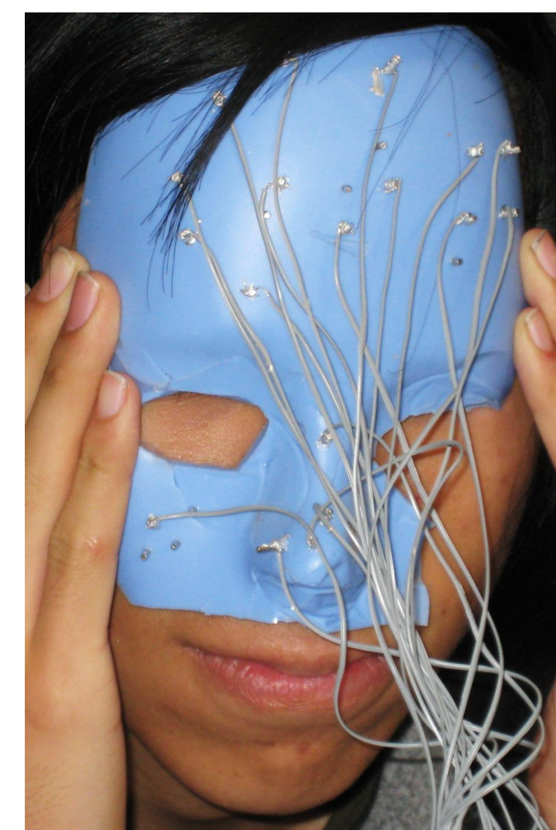
Figure 4: First prototype using a pre-made plastic mask to mold the silicone.
