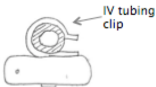
Figure 6 - Top view of the electric LED timer design showing the clipping mechanism.
