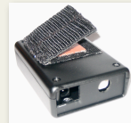
Figure 4: Velcro strap with rubber strip on the back of the final prototype
