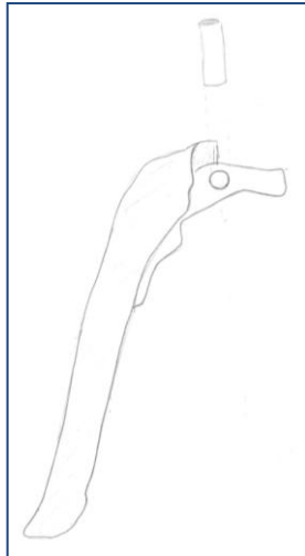
Figure 7: The components of the current stapler trigger mechanism
