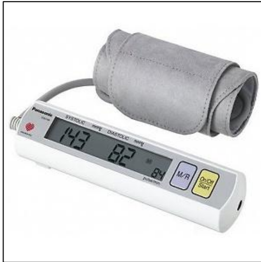
Figure 2: Blood pressure monitor that uses the oscillometric method
