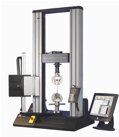
Figure 5: Image of an Instron Electromechanical System 15 .
