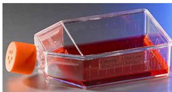
Figure 1: Static culture flasks sold by Corning (Product #3814) are frequently used to grow cells. The cells adhere to the bottom and are bathed in liquid media as shown
