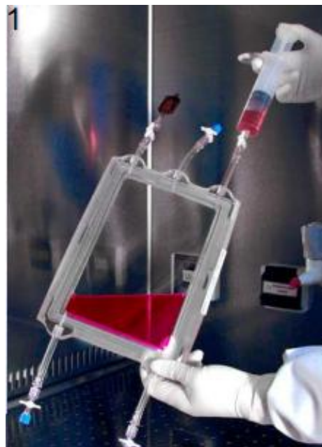
Figure 2: The CLINicell cassette provides the most competition to our design proposal in that it allows perfusion culture with adherent cells. However, the geometry of the cassette is not optimized for flow distribution, the plates are too thin, allowing oxygen permeability, and the cassette requires a high volume of media per square centimeter of growth area.
