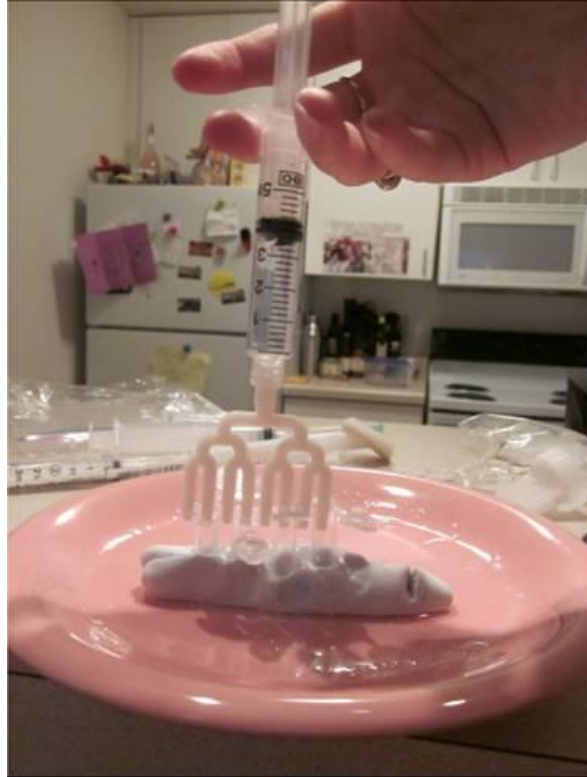
Figure 23: Setup for flow distribution using syringe.
