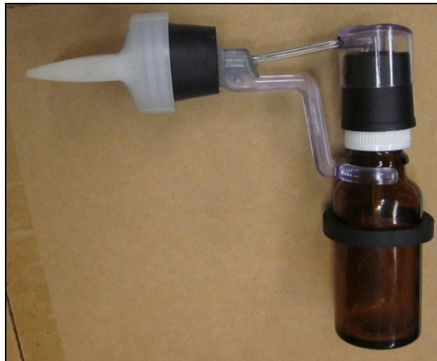
Figure 3: Current device consisting of a hollow L'Oreal hair dye comb attached to a MADomizer spray applicator from Wolfe Tory Medical using a rubber stopper.
