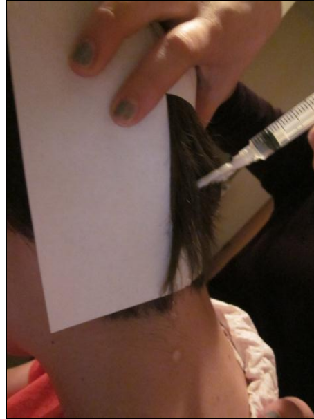
Figure 21: Setup for time trials with syringe and comb attachment. Time trials of application were done by applying 2.0 mL of water to a 50 cm 2 area on the scalp.
