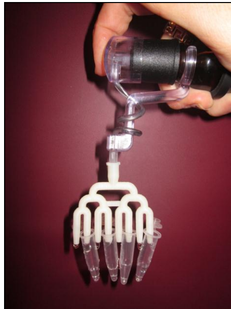
Figure 24: Fluid distribution testing was conducted using a rapid prototype of the comb tip attached to the MADomizer spray applicator.
