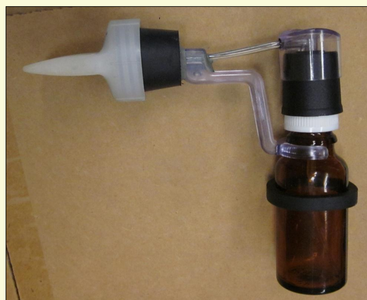
Figure 2. Current device used to apply the drug solution. It consists of a Wolfe Tory Medical, Inc. MADomizer attached to a comb via a rubber stopper.
