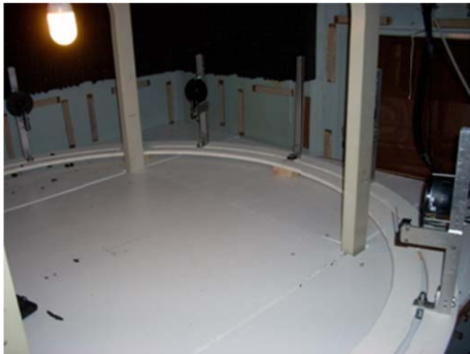
Figure 17: Perspective view of hemi circular wooden arc mounted just outside of the magnetic cube with speaker posts placed in slot cut into wood. Speakers can slide within the track for varying positions.
