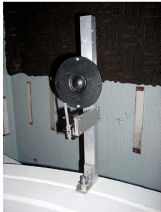
Figure 16: Individual speaker post. Shown image does not include pinch valve that will be mounted in the top set of holes
