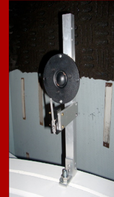
Speaker mount attached to plywood hemi circle and switch located directly in front
