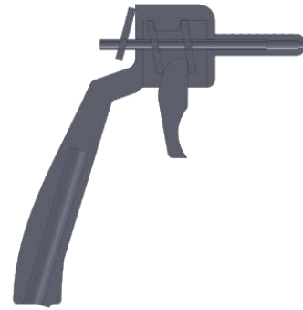
Figure 13: SolidWorks design of a slice through our prototype showing the clutch orientation.
