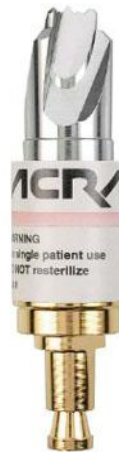
Figure 3: ACRA-CUT Smart Drill bit used in emergency neurosurgery to release pressure inside the skull. It has two offset bits and the drill only operates when pressure is applied to the inner bit. Thus, when the skull is penetrated, pressure is released from the inner bit and the bit stops operating, preventing over penetration [1].
