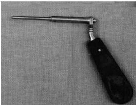
Figure 2: Drill guide used in spinal surgeries. It has a pre-set depth, but it is not able to be adjusted during operation [11].
