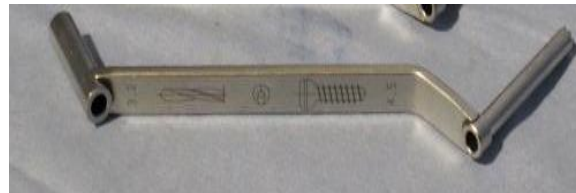
Figure 1: Drill sleeve used for most orthopedic surgeries. It contains no stopping device; it just ensures the drilling of a straight hole [7].
