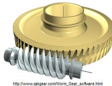
Figure 8: Worm gear example
