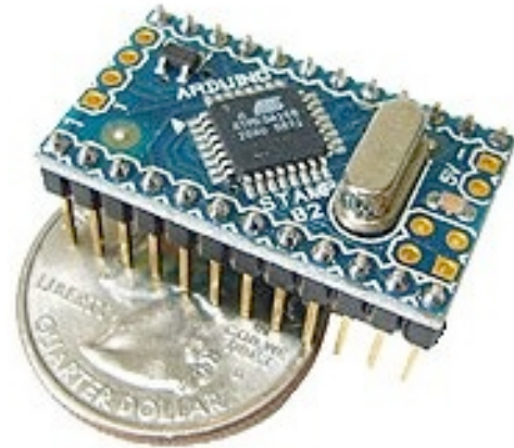
Figure 13 - The Arduino Mini will be used to program the prototype
