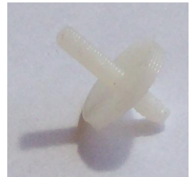
Figure 14 – Sixteen Braille pins were needed to display the time.
