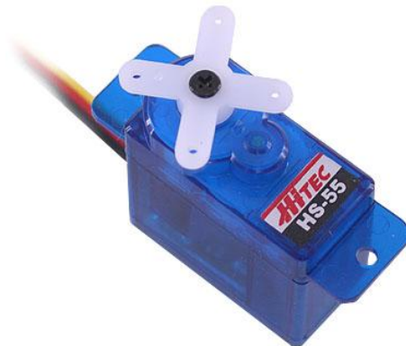
Figure 12 – Four HS-55 sub-micro servos were used to rotate the disks
