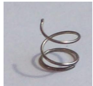
Figure 15 – Springs were cut to a fraction of their original length in order to provide the desired force.
