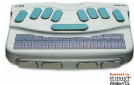
Figure 5 – HumanWare's Braille Note is used by the visually impaired to read computer screens Image courtesy of HumanWare http://www.anu.edu.au/disabilities/atproject/
