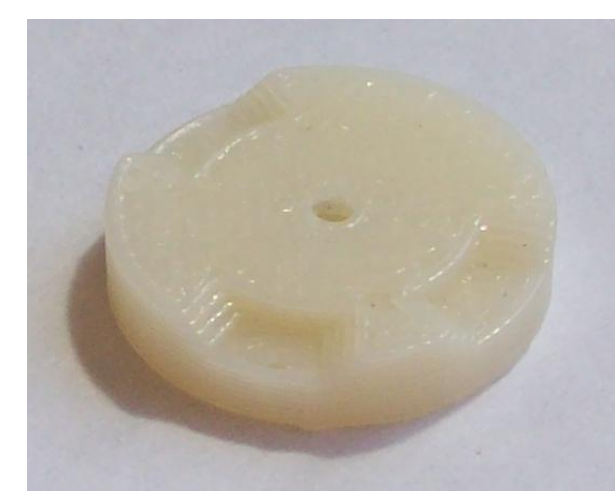
Figure 4: The rotating disks machined from ABS plastic
