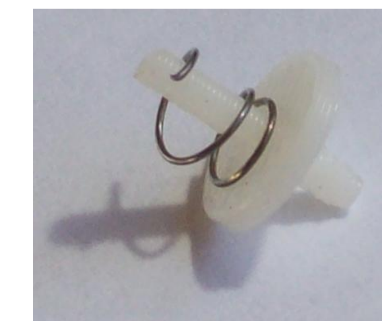
Figure 6: Each Braille pin is held in place using a compression spring
