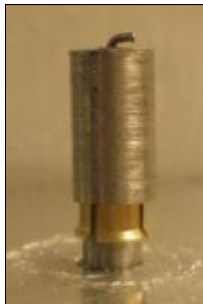
Figure 6: This is an image of the spring and sheath attachment design. This design prevents lateral displacement of the prosthesis, but it does not contain magnets to hold the prosthesis securely [5].
