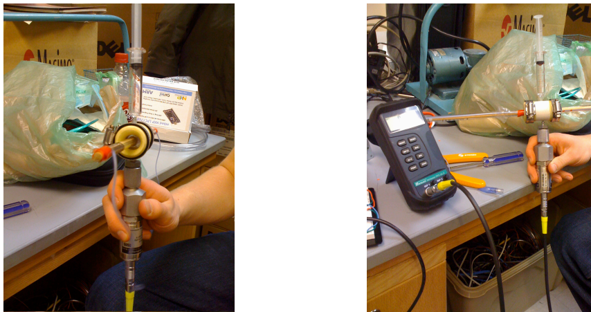
Figure 8: Pressure Tube and Measurement System
