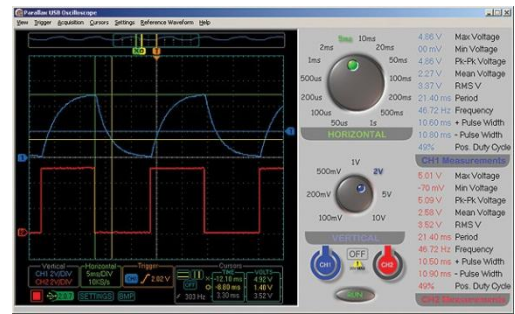
Figure 6: Graphical user interface associated with Parallax PC [d].
