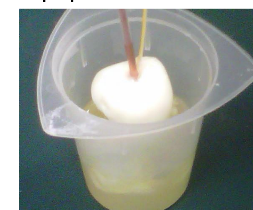
Figure 8: The final design is egg white plus albumin. The ablation zone is clearly seen.
