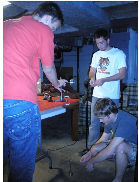
Figure 8. Using a weight set to quantitatively test the strength of the new and old levator cord design.
