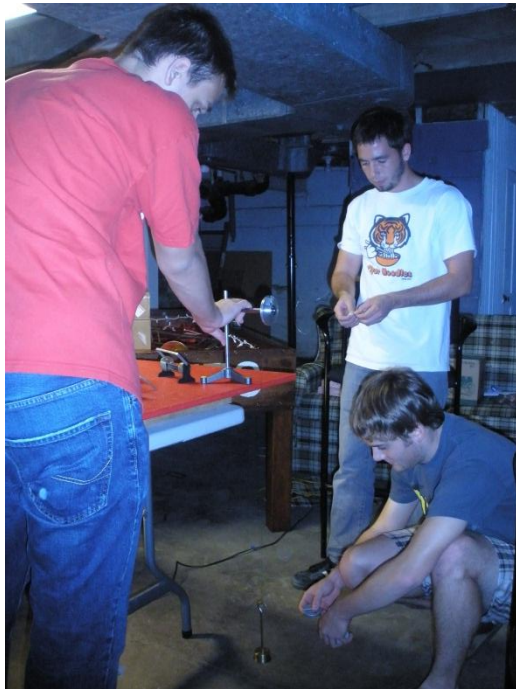
Figure 8. Using a weight set to quantitatively test the strength of the new and old levator cord design.
