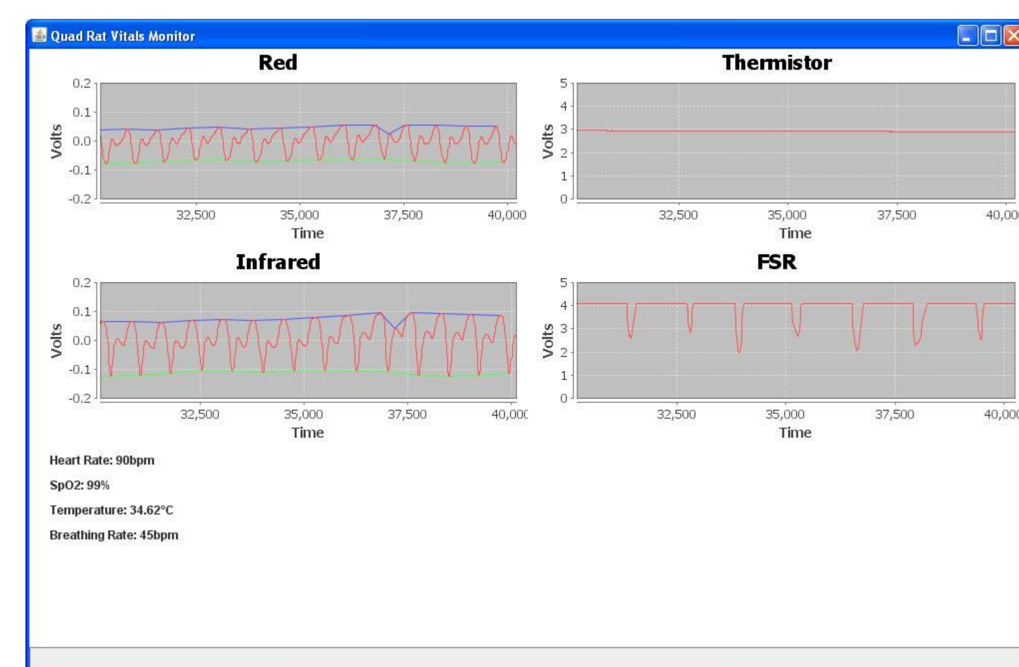
Figure 6. Graphical user interface of final product made in Java. Graphs of Red, Infrared, Thermistor and FSR are all displayed along with values of heart rate, SpO 2 , temperature and breathing rate.
