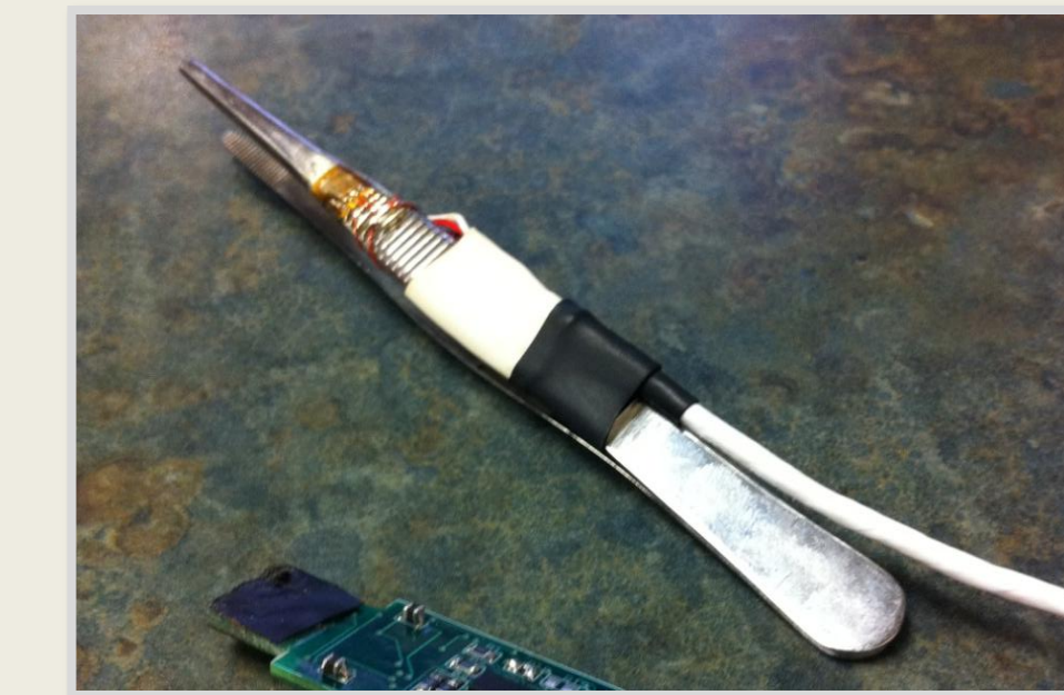
Fig. 4-8 – Final forceps, USB connection and circuitry set up for the USB bridge amplifier [7]
