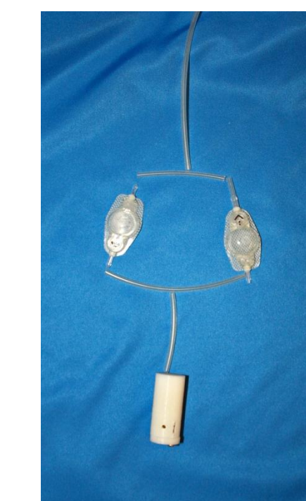
Figure 3: A photograph of the valve system. The two valves in parallel are commercial pressure differential valves while the bottom valve is the novel design.
