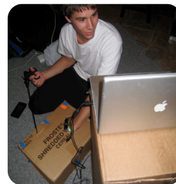
Figure 6: Josh handling a pair of graspers and using a single hand to remove cancerous kidney model from model abdomen while using web-camera as laparoscopic element
