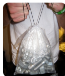
Figure 4: Seal provided by impulse heat sealer with standing about 4 kg of weight provided by metal pieces
