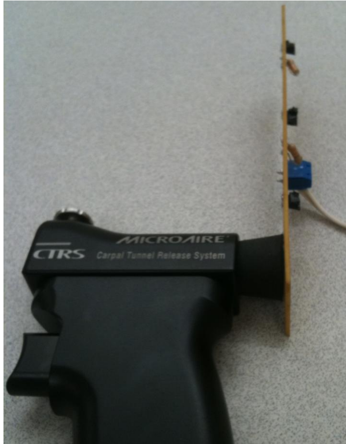
Figure 17. The circuit board is attached to the back of the endoscope shell by a rubber cap. The Wii remote views the LEDs from behind the endoscope working view.
