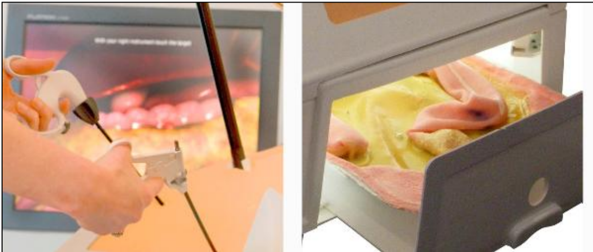
Figure 6 (left) shows the ProMIS surgical simulator utilizing virtual graphics to complete the surgery. Figure 7 (right) shows the real anatomical model included with the ProMIS system. ( http://www.haptica.com/ )
