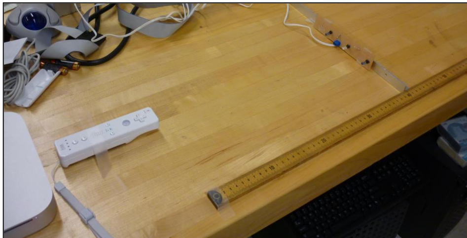
Figure 21: Testing set-up. The Wii remote is aligned with 0 on the metric ruler, and the circuit board with LEDs was moved along in 1 cm intervals.
