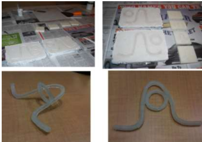
3 rd generation molds and silicone prototypes employing circular bar in two configurations
