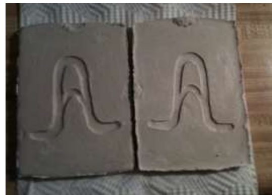
Figure 9: Dental stone mold cavity
