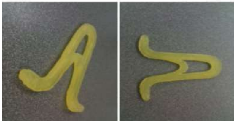
3 rd generation prototypes in 70A (top) and 70A/30A 50:50 mix (bottom)
