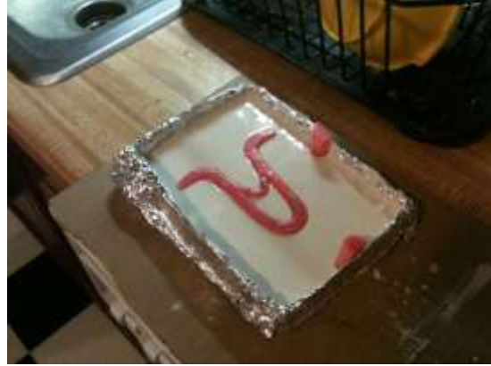
Figure 8: Wax mold in dental stone
