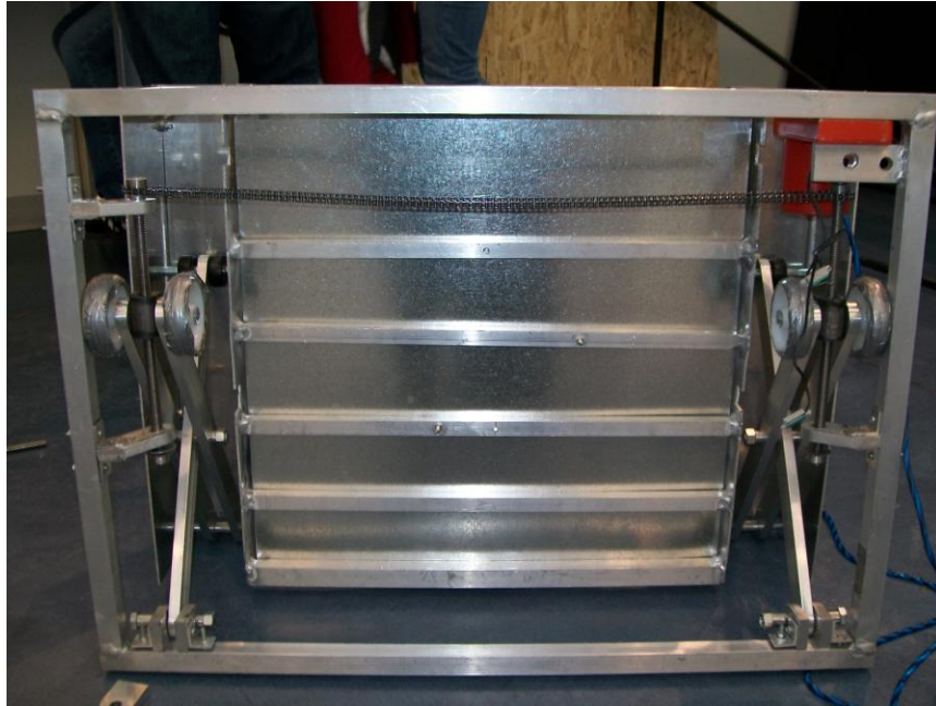
Figure 13 - Photo of lifting mechanism of final device
