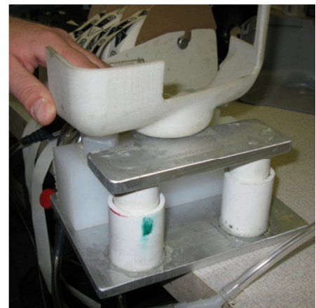
Figure 6: Template and Spring System The template is fastened to the spring support system. The spring allow for the template to move up and down.
