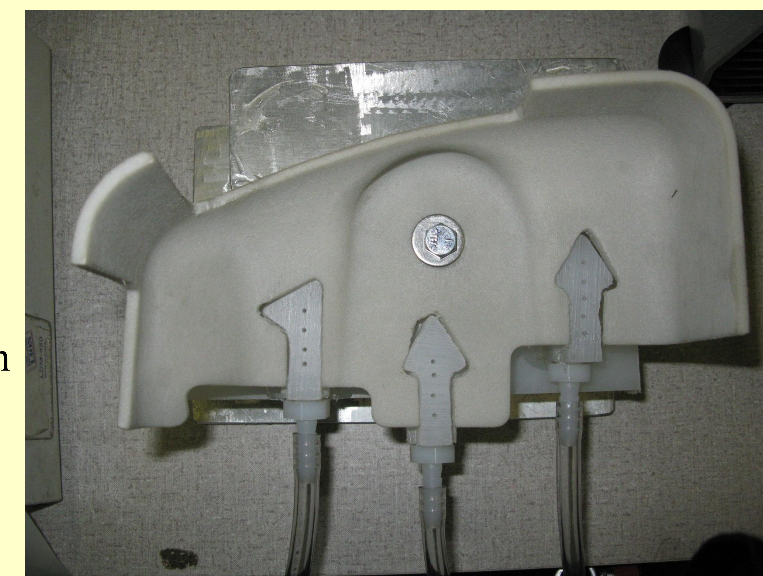
Figure 3 (left)- Vacuum and Valves. The arrow pedestals are connected via polyethylene tubing to a vacuum pump. The vacuum can create up to a 25 mmHg vacuum pull. To utilize the full vacuum potential for each pedestal, valves are incorporated to isolate the vacuum.
