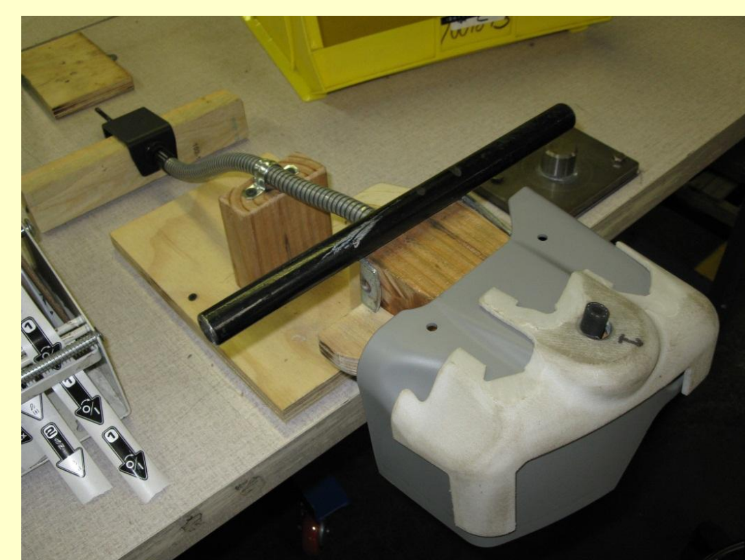
Figure 1 (left)- Current Method. The engine shroud (dark grey) is mounted on a fixture with the template (white) placed on top. The employee then places three stickers (seen on far left) in the slots cut into the template. The stickers need to be accurately placed and without wrinkles or bubbles
