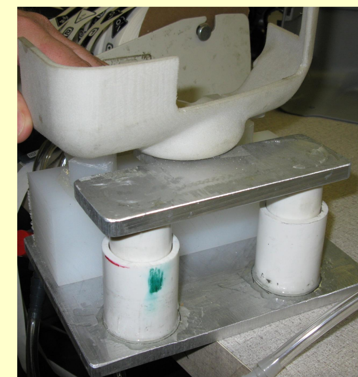
Figure 3 (left)- Vacuum and Valves. The arrow pedestals are connected via polyethylene tubing to a vacuum pump. The vacuum can create up to a 25 mmHg vacuum pull. To utilize the full vacuum potential for each pedestal, valves are incorporated to isolate the vacuum.
