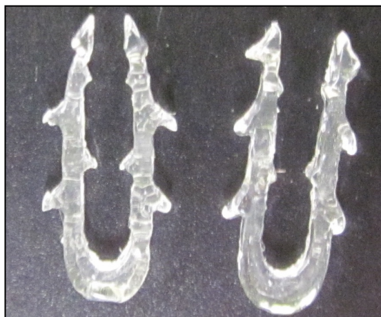
Figure 23: Picture of staples after being cut with the laser cutter
