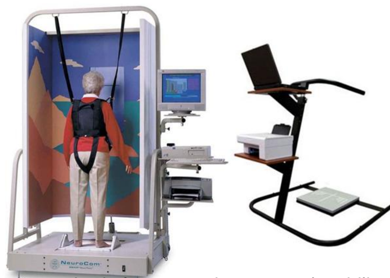
Figure 1: Current methods for measuring postural stability, NeuroCom® Balance Manager 4 (left), and the Clinical Grade Force Plate 5 .
