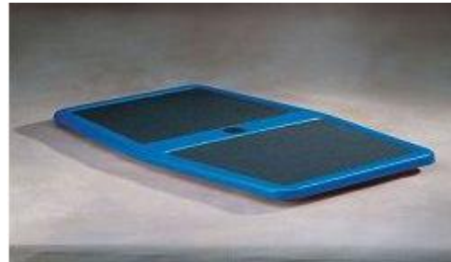
Figure 7: The BEEP Board is design after a first class lever where any shift in weight would produce an audible signal. [13]
