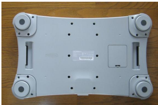
Figure 5: A force plate displayed where the four pedestals are with the transducers in them. [10]
