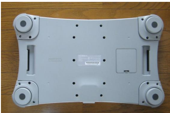
Figure 5: The dorsal side of a Wii Board displays the four legs each with a transducer. [13]
