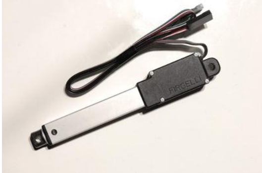
Figure 6: Linear Servomotor from Firgelli Technologies Inc. This motor is 16mm in width, the stroke length is 140mm, and the maximum force generated is 30N. Source: www.firgelli.com
